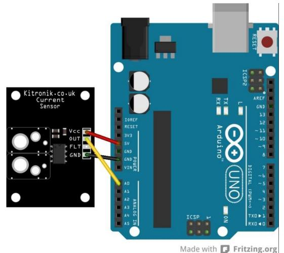
This board is very simple to connect to the Arduino. To begin measuring current with the current sensor connect the pins on the breakout board to your Arduino as described in the table below.
